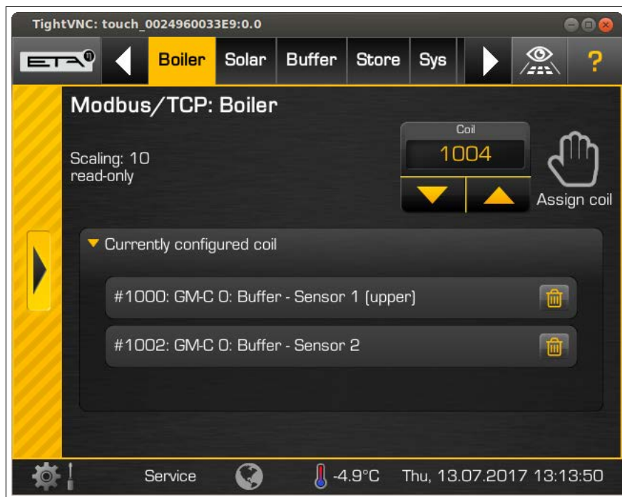
Figure 8: Register configuration screen on the ETAtouch for software versions \geq x.36.0 .
